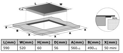
Under any circumstances, make sure the Induction cooker hob is well ventilated and the air inlet and outlet are not blocked. Ensure the Induction cooker hob is in good work state. As shown below
